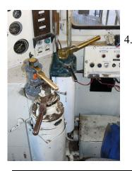
Install the console handles (if any have been removed), Throttle (select to IDLE) Reverser (select to NEUTRAL), Automatic (select to RUN), Independent (select to full application -"against-the-spring")
